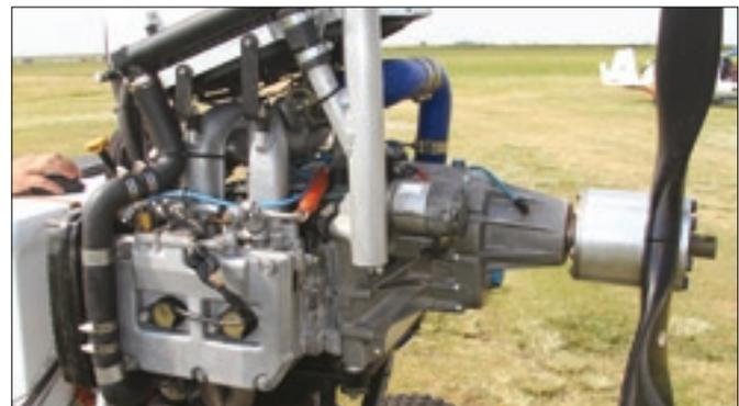
**The Subaru engine with Garret turbocharger and three-bladed propeller**
