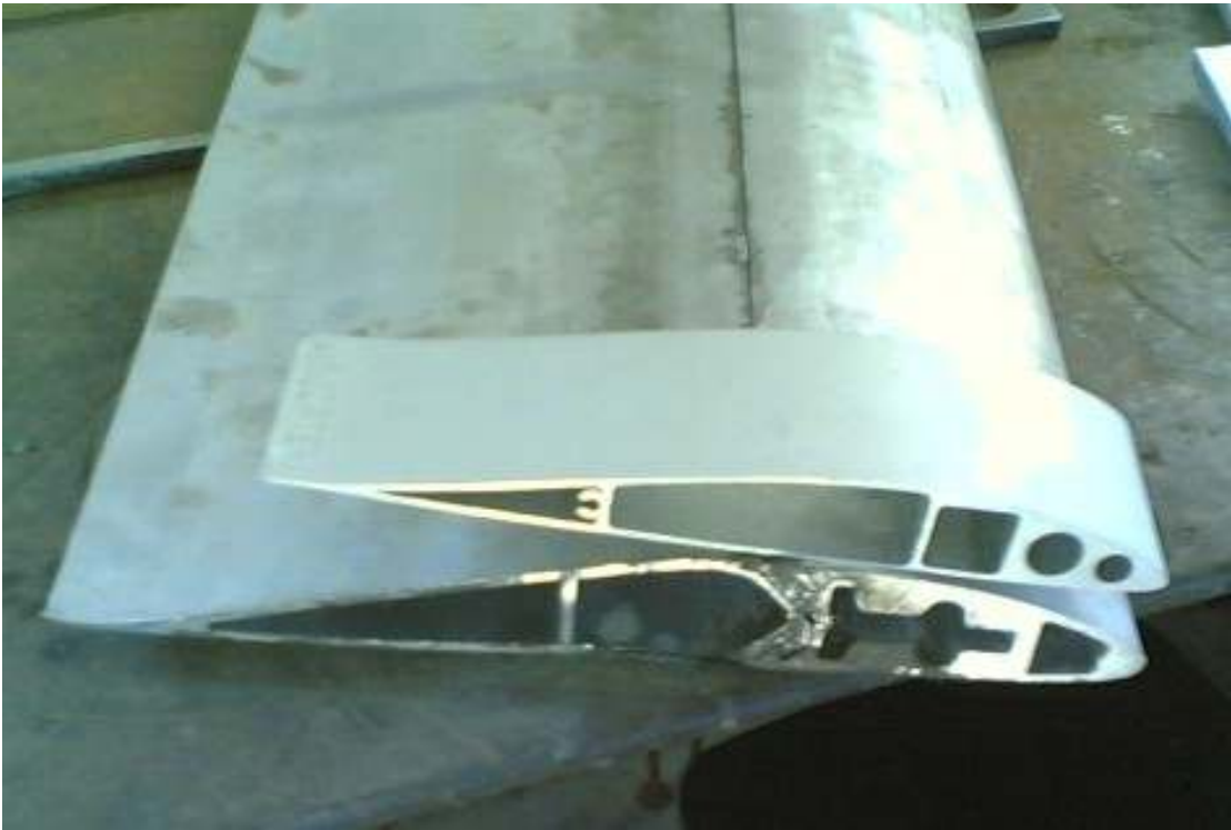
New 250 mm rotor blades compared to existing 220 mm units
