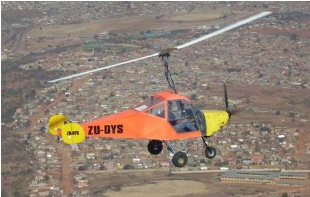
Kriek MKIIB with new tricycle undercarriage
