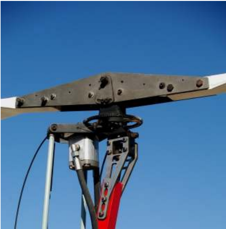
Rotor head with adjustable pitch mechanism and hydraulic motor
