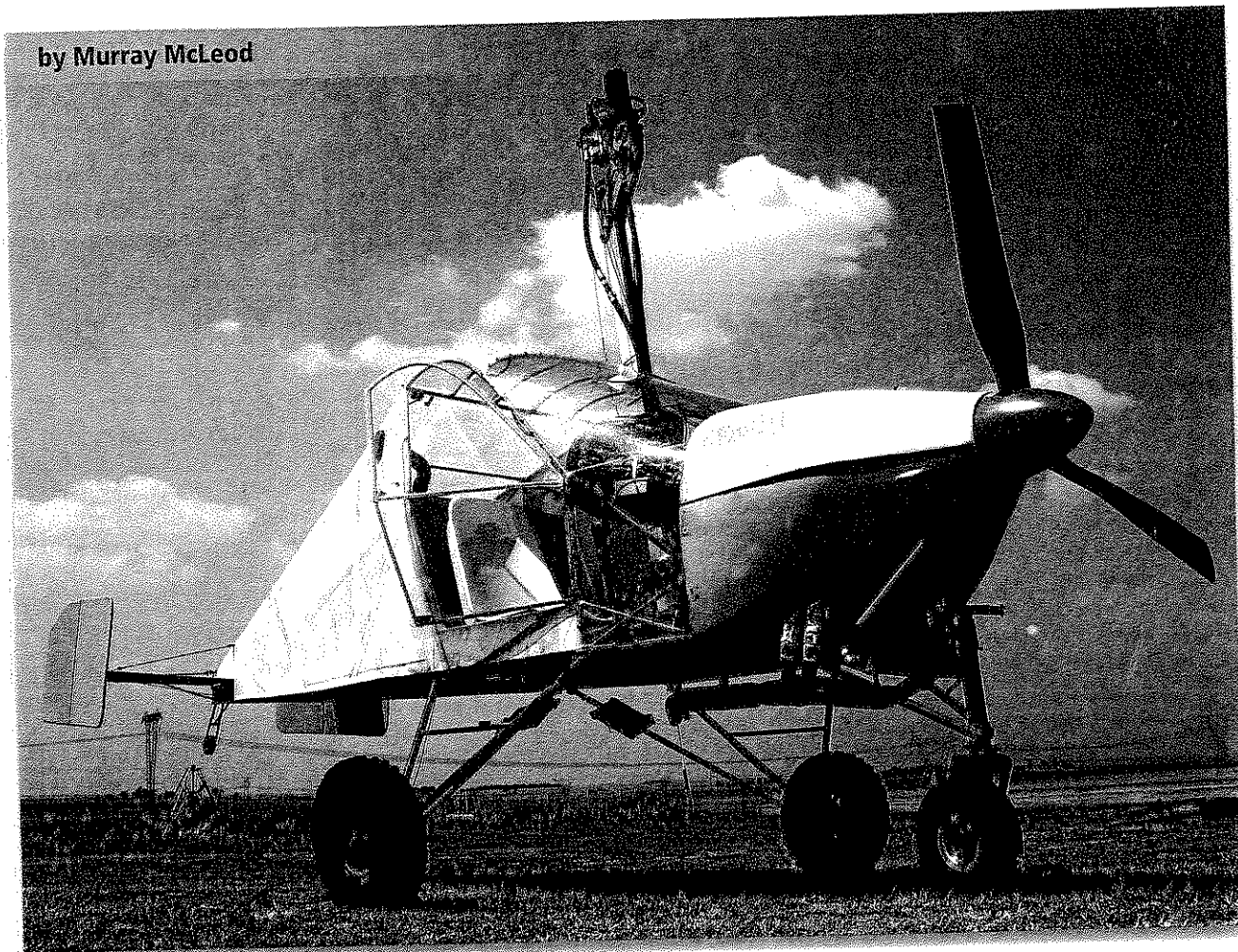
New and unflown Kriek-4 is powered by a flat-four Subaru engine.
